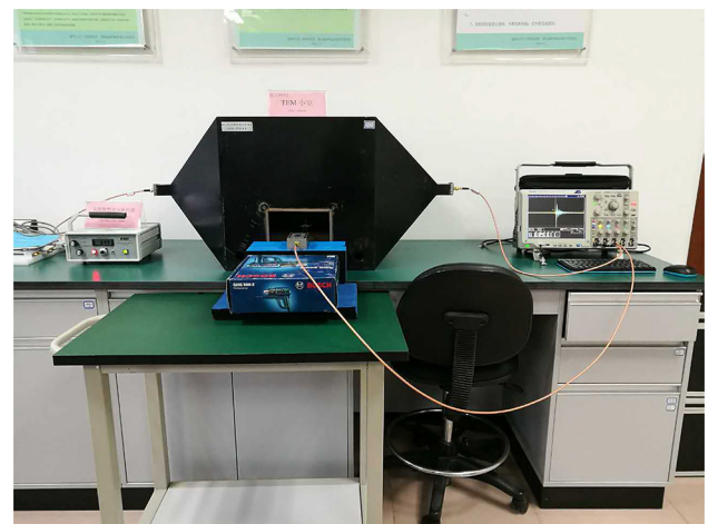
Fig. 6 Experimental setup for the 300 MHz TEM cell calibration
