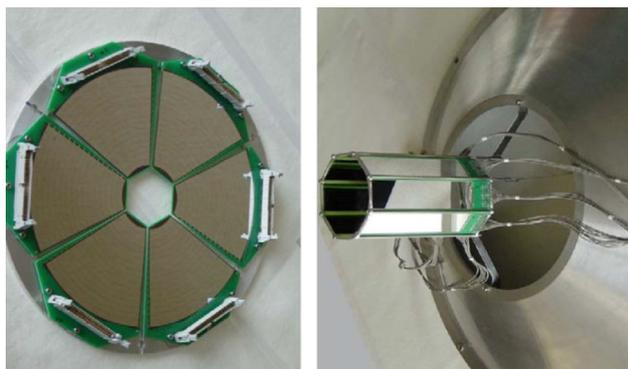
**Fig. 10** (Color online) The SiHyBall annular detector (left) and the octagonal barrel (right). This figure is from [37]
