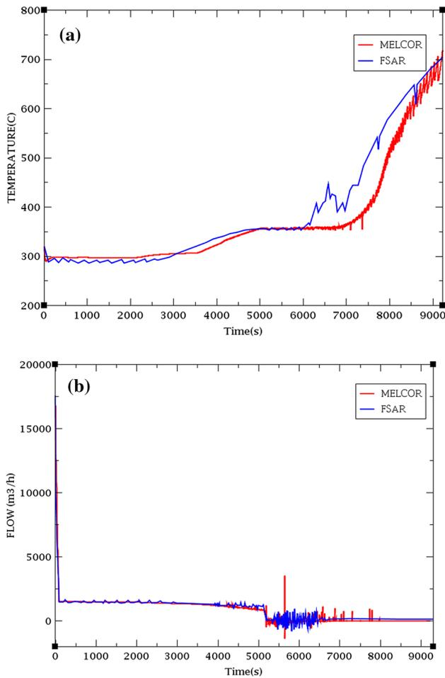
**Fig. 7** (Color online) **a** Hot leg temperature, **b** coolant flow rate in the primary side
