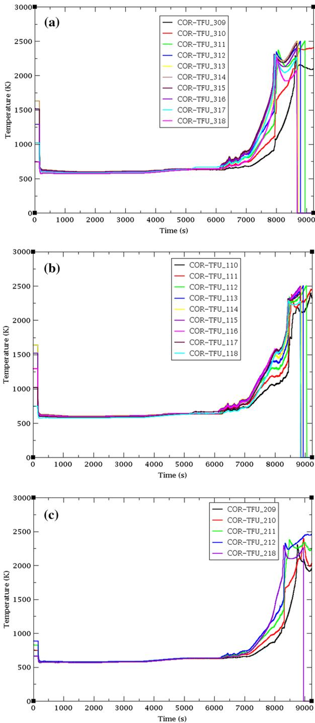
**Fig. 9** (Color online) **a** Fuel temperature in the ring with the highest power (ring 3), **b** temperature of the fuel rods in ring 1, **c** temperature of the fuel rods in ring 2
