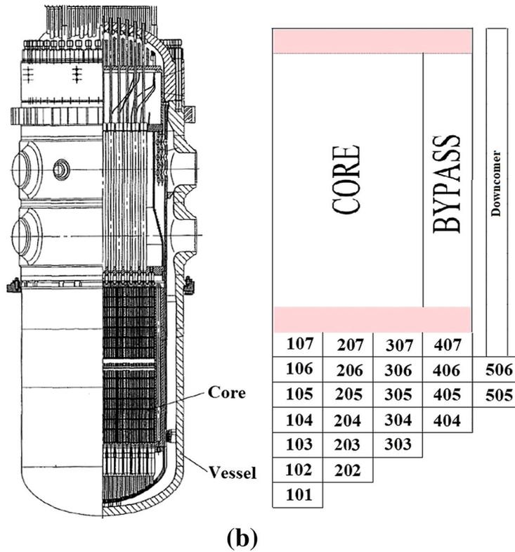
**Fig. 3** a Nodalization of the SG and the secondary side of the power plant, b nodalization of the core and the lower plenum
