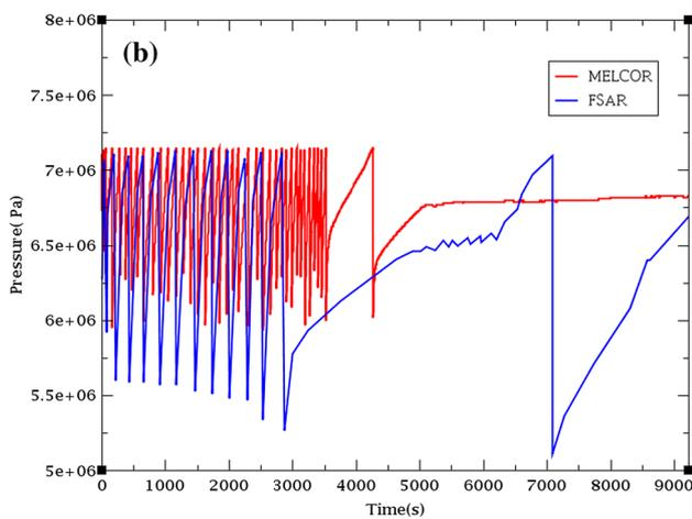
Fig. 5 (Color online) a Water level in a steam generator, b pressure of the steam generator
