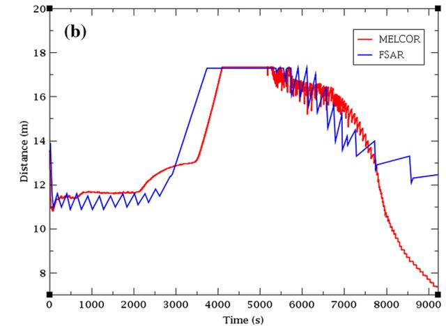
Fig. 6 (Color online) a Pressure in the PRZ, b water level in the PRZ
