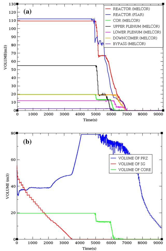
**Fig. 8** (Color online) **a** Total volume of water in the reactor's components, **b** coolant volume in core, steam generator and PRZ
