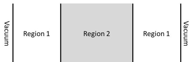
Fig. 5 Geometry of the modified OECD / NEA one-dimensional slab benchmark
