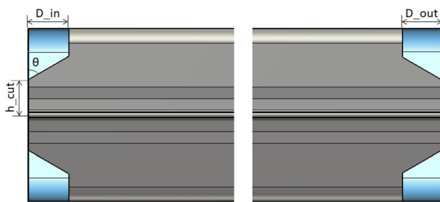
Fig. 10 Design diagram of undercuts
