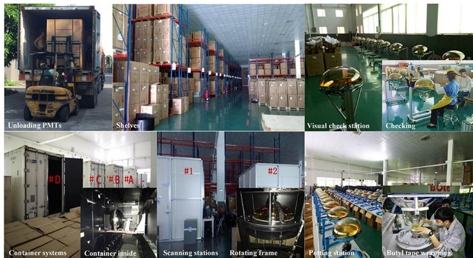
sampled to retest for performance using container systems #A, #B, and #D. The retested and qualified LPMTs were then stored on the shelf again, pending subsequent transport to the JUNO site. It was necessary to register all the LPMTs again before they left the warehouse.
