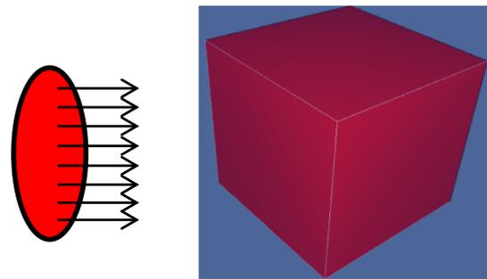
**Fig. 1** Disk gamma-ray source and the cubic concrete sample simulated using the MCNPX code (Color online)
