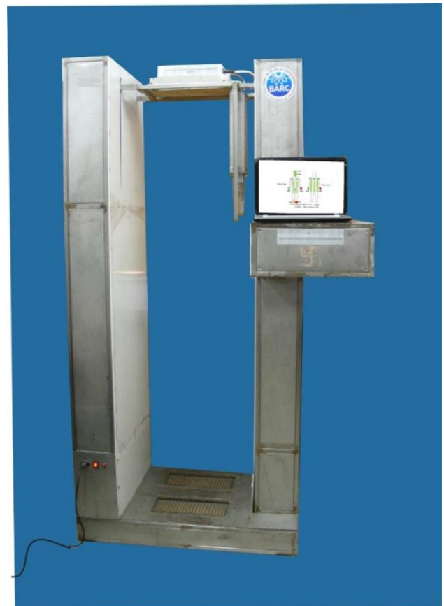
Fig. 1 (Color online) Plastic scintillator detectors based whole body contamination monitoring system
