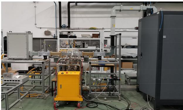
**Fig. 7** (Color online) SHINE 1.3 GHz FPC high RF power test system
