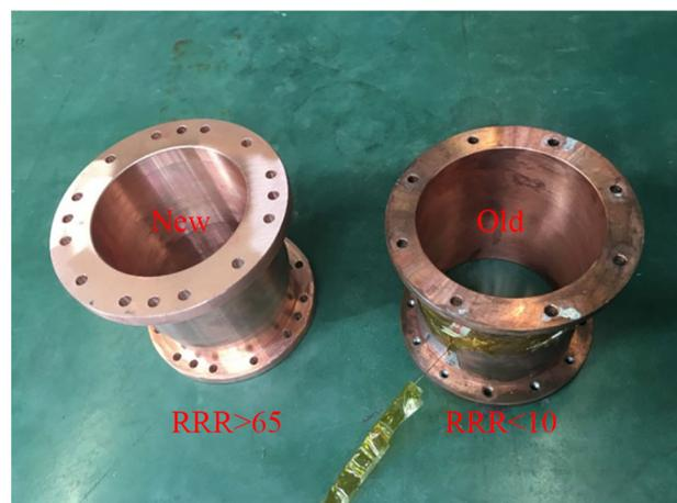
Fig. 24 (Color online) Photograph and RRRs of the new and old copper cylinders
