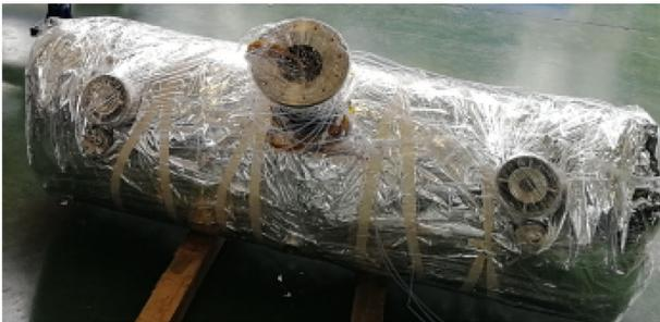
**Fig. 10** (Color online) 4.2 K helium vessel with superinsulation
