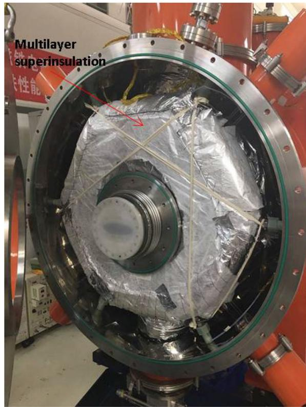
**Fig. 19** (Color online) Photograph of multilayer superinsulation wrapping
