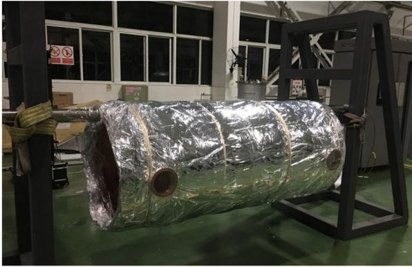
**Fig. 9** (Color online) 60 K thermal shield with superinsulation
