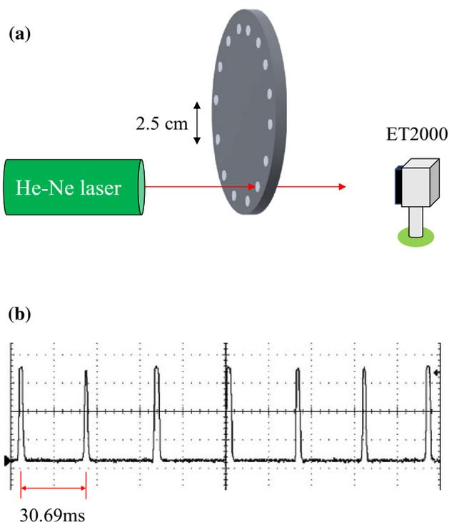
**Fig. 2** (Color online) **a** This irradiation duration was measured using a He-Ne laser, a photodiode (ET2000), and an oscilloscope. **b** The time interval between two holes 2.5 cm apart is approximately 30.69 ms. The irradiation time on each CR-39 detector was deduced to be approximately 12.5 ms
