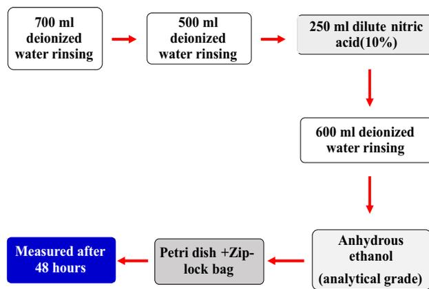
**Fig. 3** (Color online) Post-processing of the CR-39 solid-state track detector
