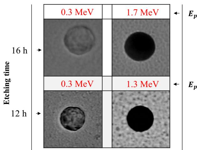
**Fig. 5** When the diameters are the same, the proton energy level can be distinguished according to the gray level of the track
