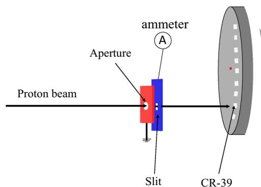
**Fig. 1** (Color online) Layout of experimental setup. The aperture has a diameter of 1 cm, and the slit has a width of 0.439 mm
