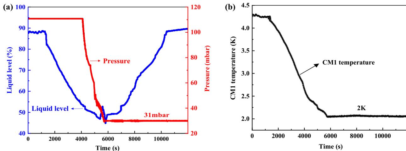
**Fig. 21** (Color online) **a** Relationship between the liquid helium level and pressure over time when the CM1 cooled down from 4 to 2 K; **b** CM1 temperature cool-down curve
