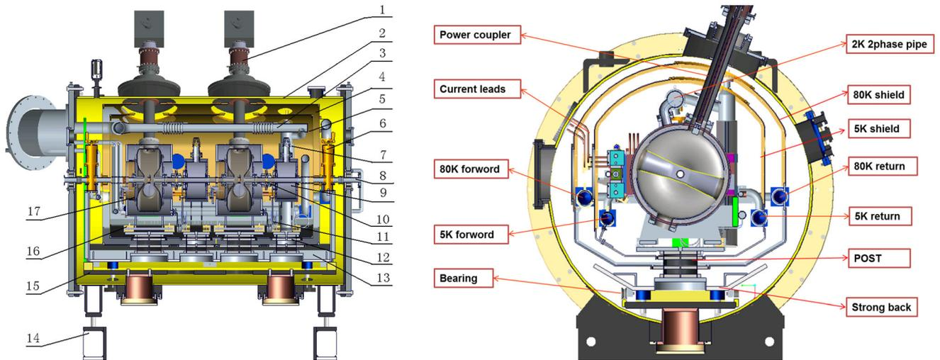
**Fig. 14** (Color online) TCM cryomodule diagram. 1—coupler; 2—vacuum cylinder; 3—two-phase pipe of 2 K pump group; 4—80 K liquid nitrogen shield; 5—5 K helium shield; 6—vacuum gate valve; 7—level gauge pipe assembly; 8—beam tube; 9—superconducting magnet + current lead; 10—low temperature BPM; 11—cool-down/
