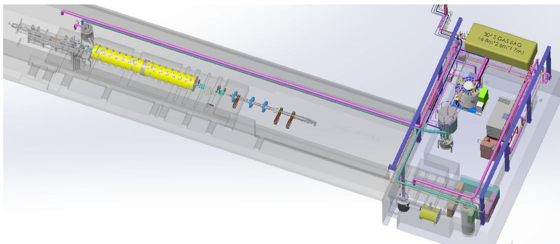
Fig. 4 (Color online) Three-dimensional diagram of the ADS Inject I cryogenic system
