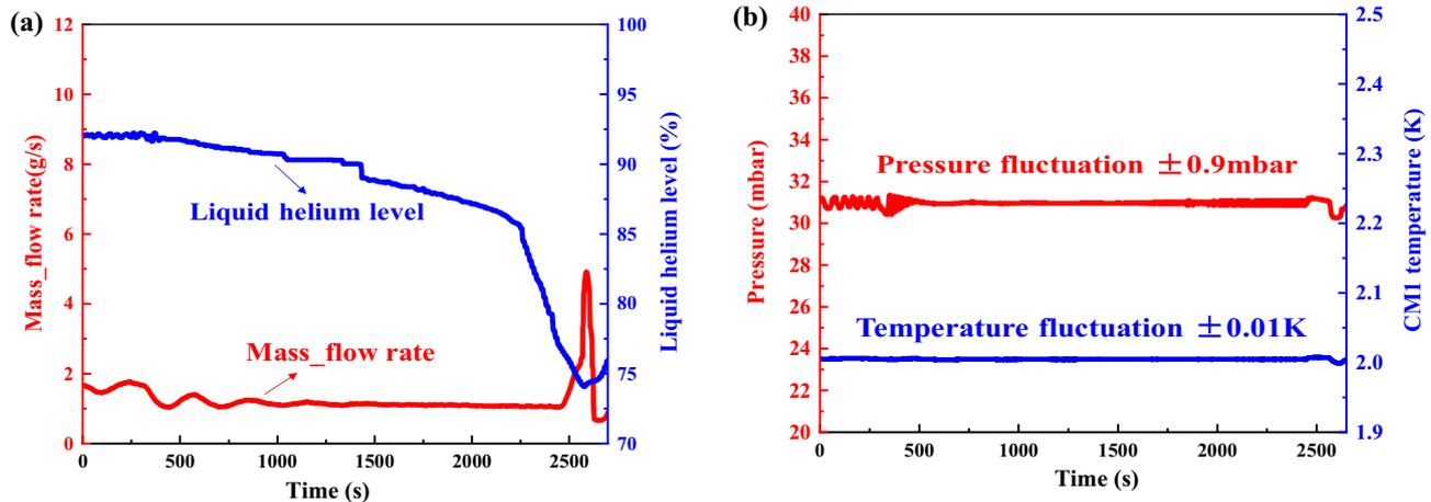
**Fig. 19** (Color online) CM1 static heat leakage measurement curve; **a** the relationship between the liquid helium level and mass flow rate versus time; **b** CM1 temperature and pressure curve
