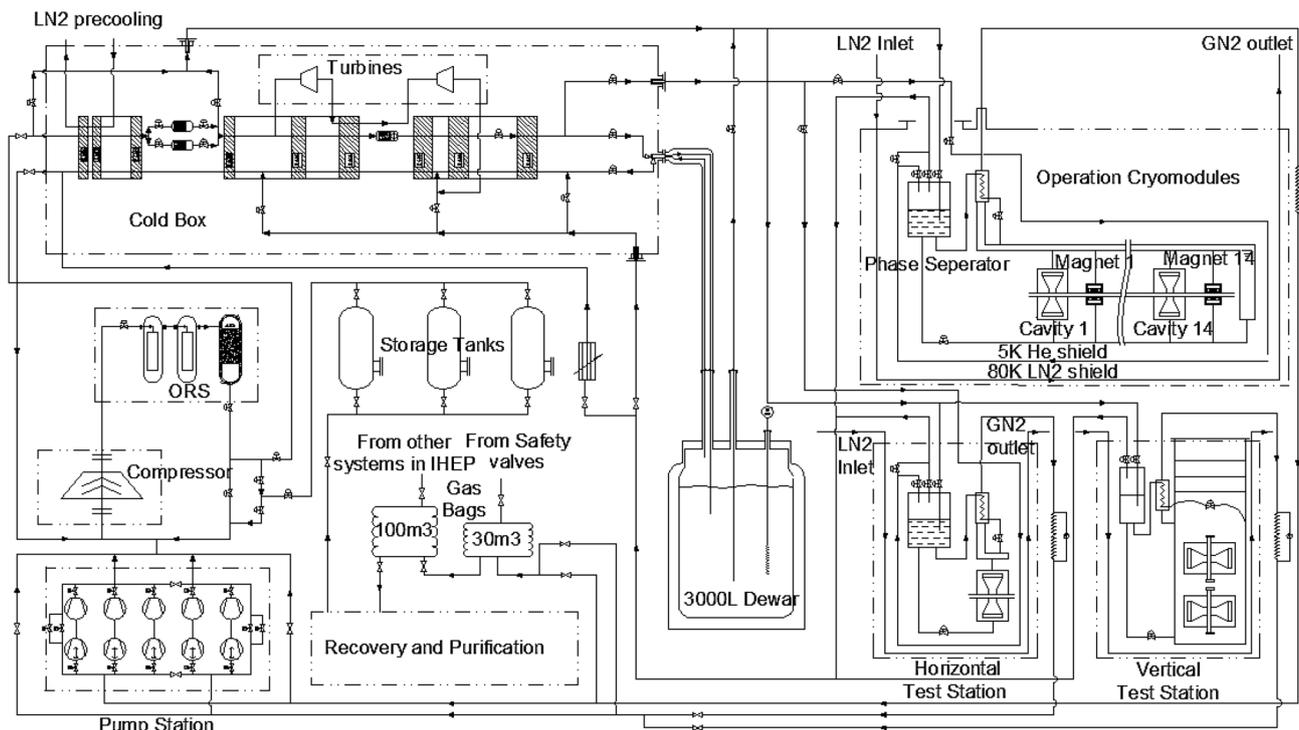
Fig. 3 PFD diagram of the ADS Injector-I cryogenic system
