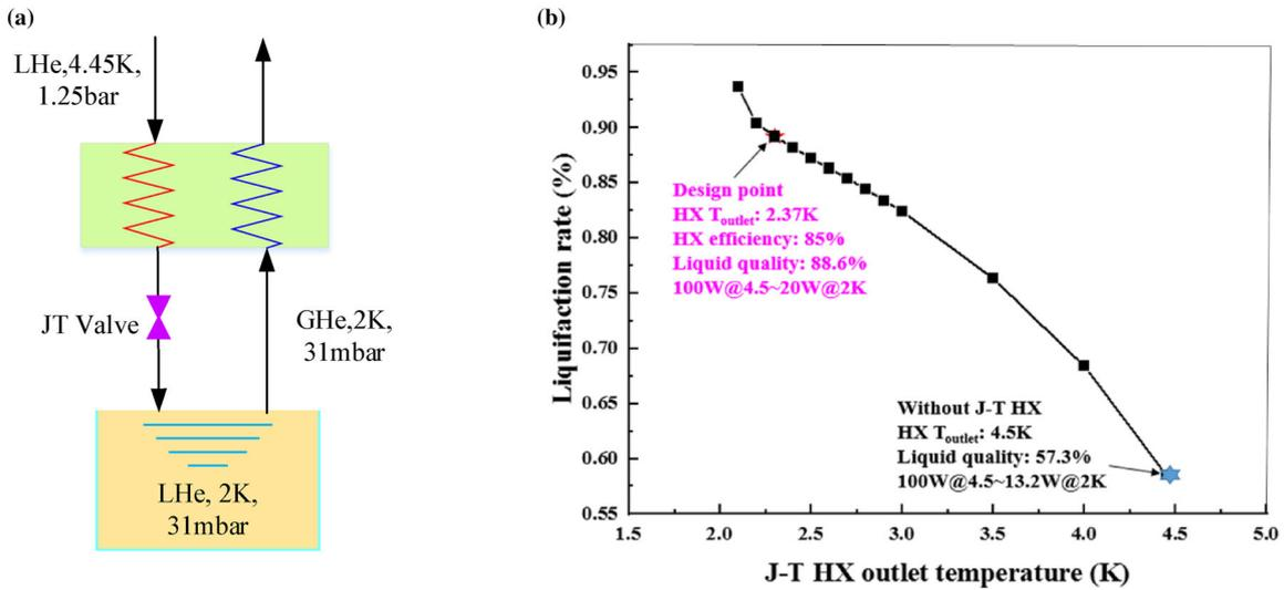
Fig. 10 (Color online) Obtaining 2 K through a J-T heat exchanger and J-T valve
