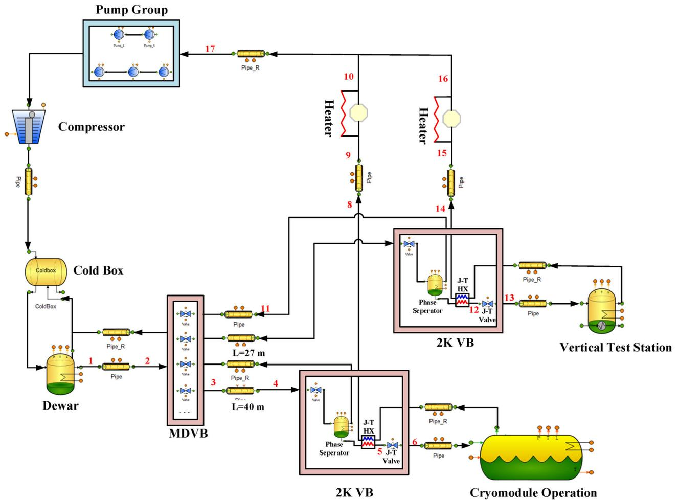
Fig. 5 (Color online) Process calculation model
