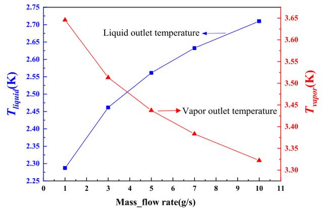
Fig. 13 Relationship between the liquid and vapor outlet temperature and the mass flow rate
