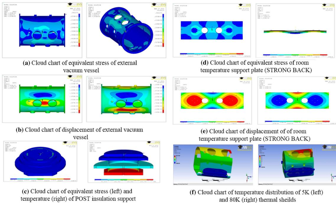
**Fig. 15** (Color online) Finite-element analysis of key components with ANSYS
