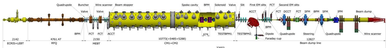
Fig. 2 (Color online) General layout of ADS Injector-I
