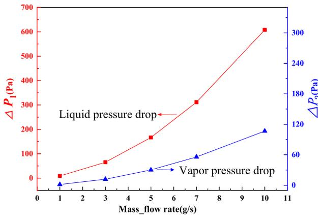
Fig. 12 Relationship between the liquid and vapor pressure drop and the mass flow rate
