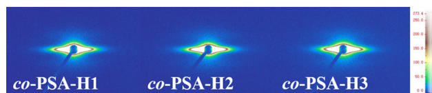
Fig. 4 (Color online) SAXS patterns of heat-drawn co -PSA fibers at different jet draw ratios ( \lambda_1 increases from 5.5 to 8.5, \lambda_2 = 2 )
