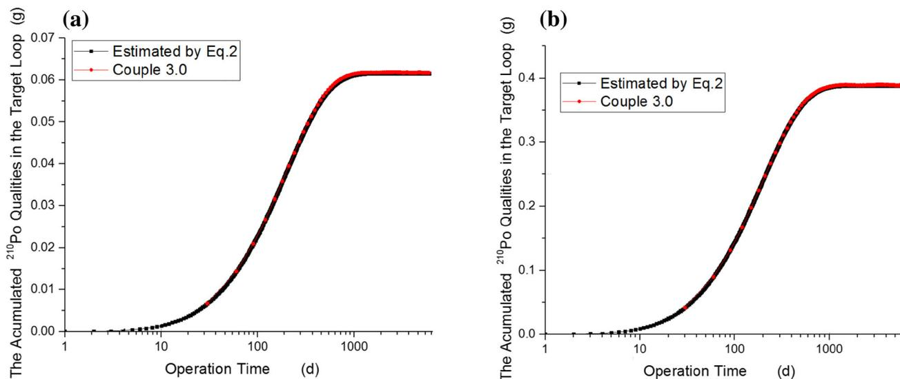
Fig. 7 (Color online) Accumulation of <sup>210</sup>Po for the LBE spallation target operated independently (a) and coupled with reactor (b)
