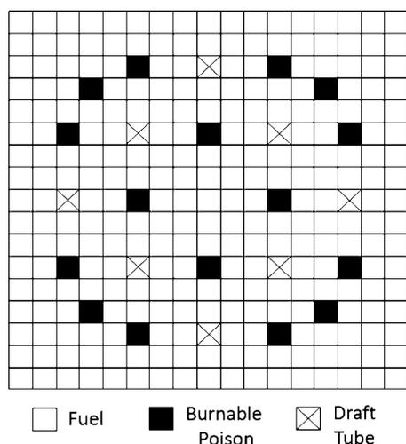
Fig. 8 Calculation model of the burnable poison
