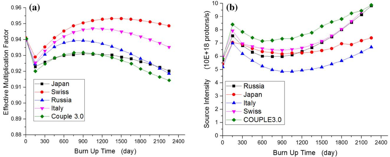
**Fig. 5** (Color online) Changes of effective multiplication factors (a) and the beam intensity (b) during burnup
