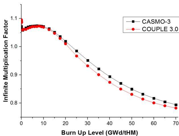
**Fig. 9** (Color online) Burnup behavior of the infinite multiplication factor
