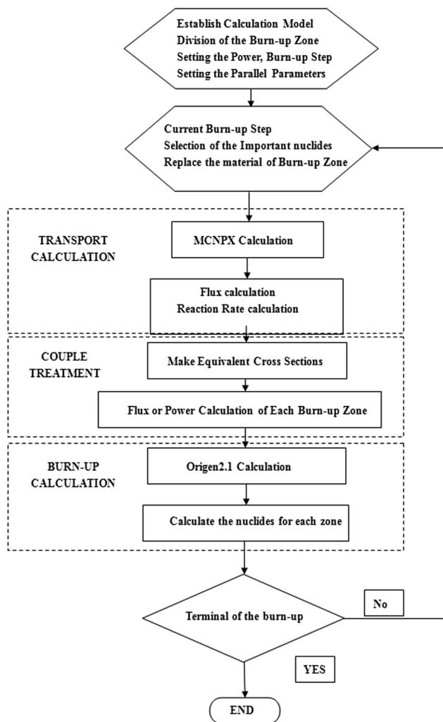
Fig. 1 Calculation process of neutron irradiation in COUPLE3.0
