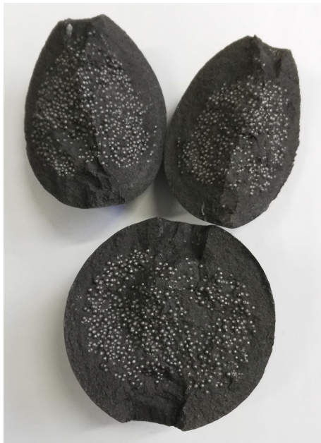
Fig. 10 Cracked pseudo-element after crushing load test
