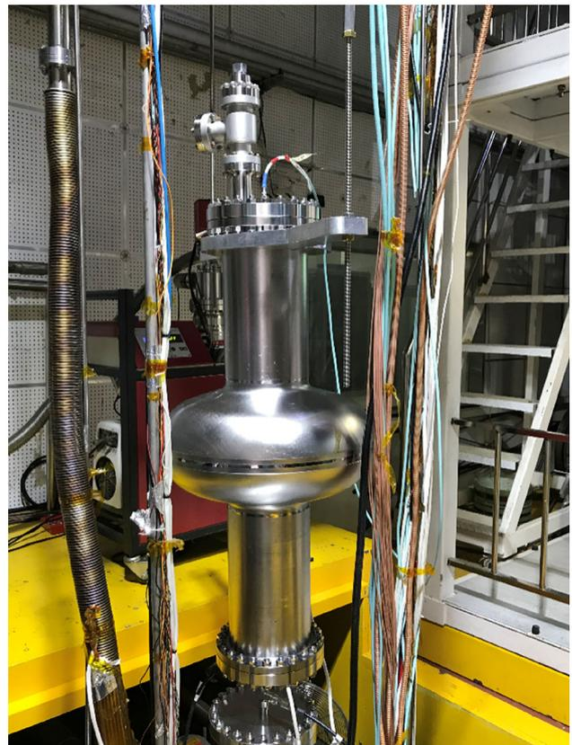
**Fig. 2** (Color online) Site photograph of vertical test of 650 MHz single-cell cavity
