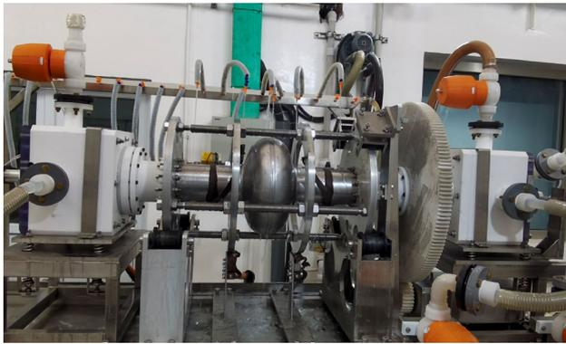
**Fig. 4** (Color online) Setup of EP process of 650 MHz single-cell cavity
