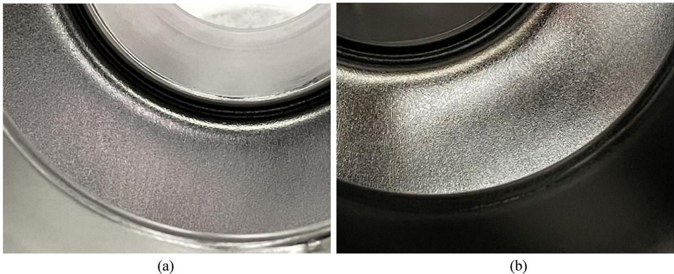
**Fig. 8** (Color online) Inner surface of 650S4 (cell). **a** Before the 2nd EP; **b** after the 2nd EP
