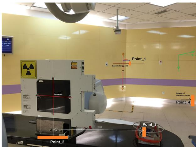
**Fig. 5** (Color online) Treatment room, MWPC, and radiation measurement dosimeter layout and geometry
