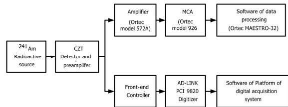
Fig.7 The block diagram of the experimental apparatus.
