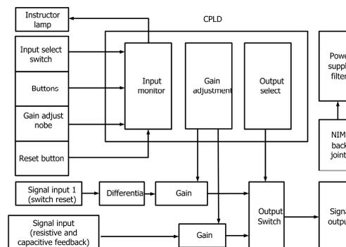
**Fig.1** Structure diagram of the front-end controller.
