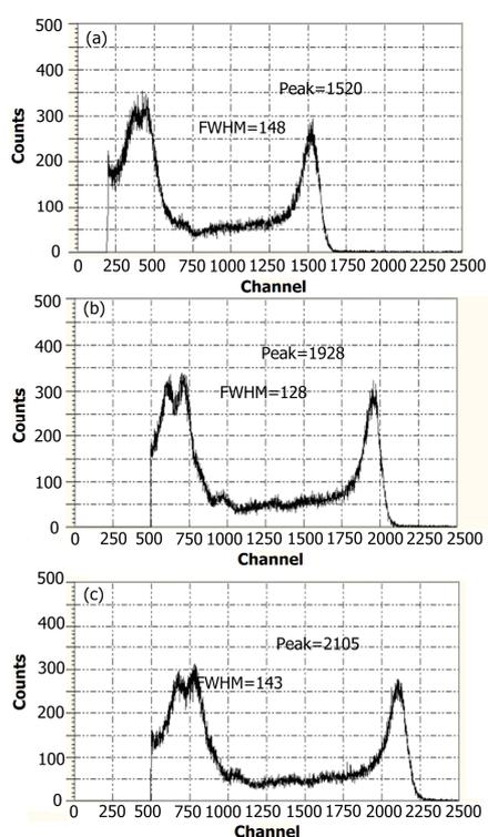
**Fig.8**  $\gamma$ -ray energy spectra of  $^{241}\text{Am}$  with CZT detector under different conditions. (a) The spectrum acquired by conventional analog system. (b) The spectrum acquired by digital acquisition system with TTF algorithm. (c) The spectrum acquired by digital acquisition system with AFTF algorithm.
