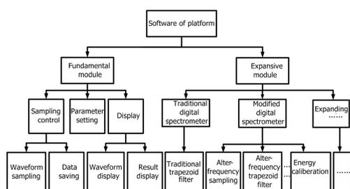
Fig.2 The structure diagram of the platform software
