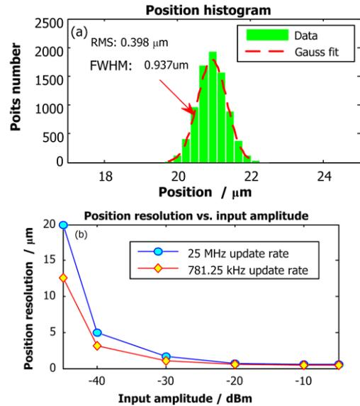
**Fig.13** Test results of position measurement. (a) Histogram of position measurement results (input amplitude:  $-10$  dBm, bandwidth:  $780$  kHz), (b) Position resolution with different input signal amplitudes.
