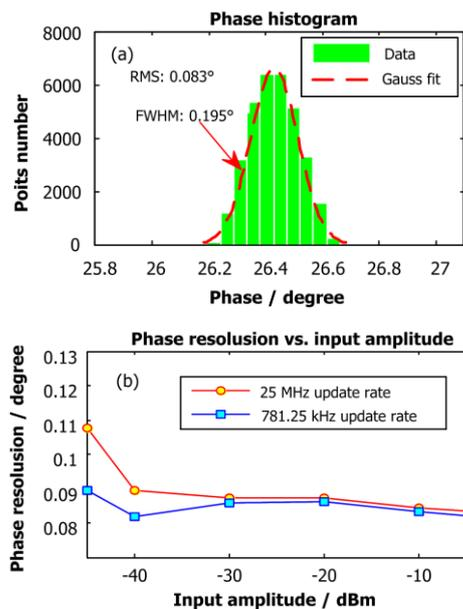
**Fig.12** Test results of Phase measurement. (a) Histogram of phase measurement results (input amplitude:  $-10$  dBm, bandwidth:  $780$  kHz), (b) Phase resolution with different input signal amplitudes.
