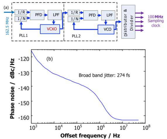
**Fig.7** Clock generation circuits design and simulation. (a) Block diagram of the clock generation circuits, (b) Phase noise simulation results of the clock generation circuits.
