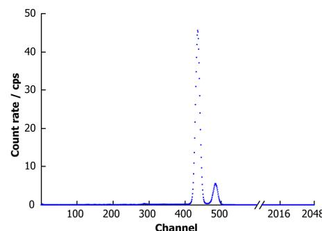
**Fig.8** Measuring result of <sup>55</sup>Fe with digital S-K filtering technique.
