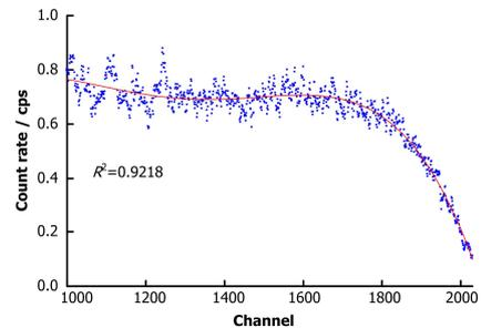
**Fig.12** Spectrum from 1000 to 2030 channel with digital S-K smooth filter.
