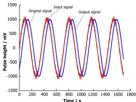
Fig.3 Digital S-K filtering waveforms for sinusoidal signal
