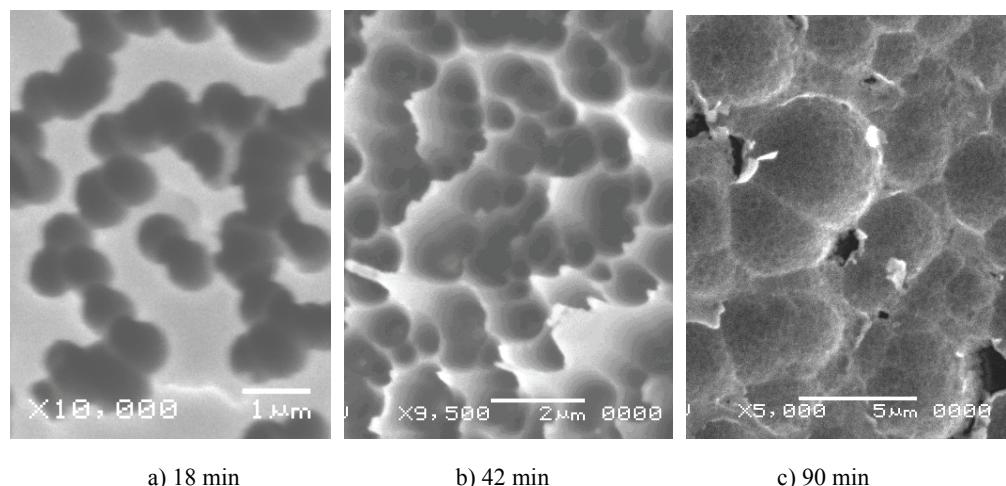
**Fig.2** Nuclear pores in polyester membranes etched in different minutes and coated with Ag of  $128 \mu\text{g}/\text{cm}^2$ .
