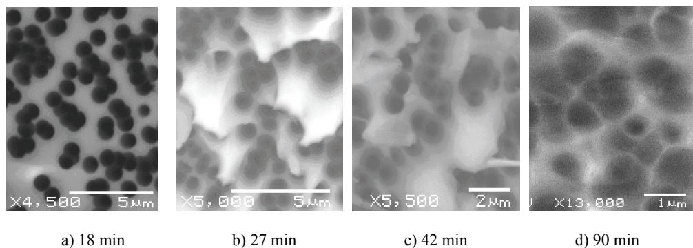
**Fig.1** Nuclear pores of different sizes in polyester membranes etched for 18–90 min in 6.0 mol/L NaOH at 65°C.
