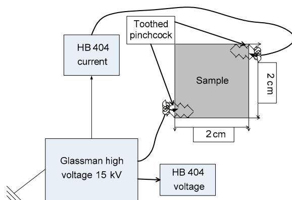
**Fig. 3** Schematic diagram of the current measurement.
