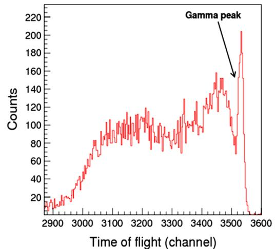
Fig. 6. (Color online) Time-of-flight (TOF) spectrum for neutrons and gamma rays.
