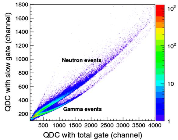
Fig. 5. (Color online) A typical result of the pulse shape discrimination (PSD) in a BC501A liquid scintillator.
