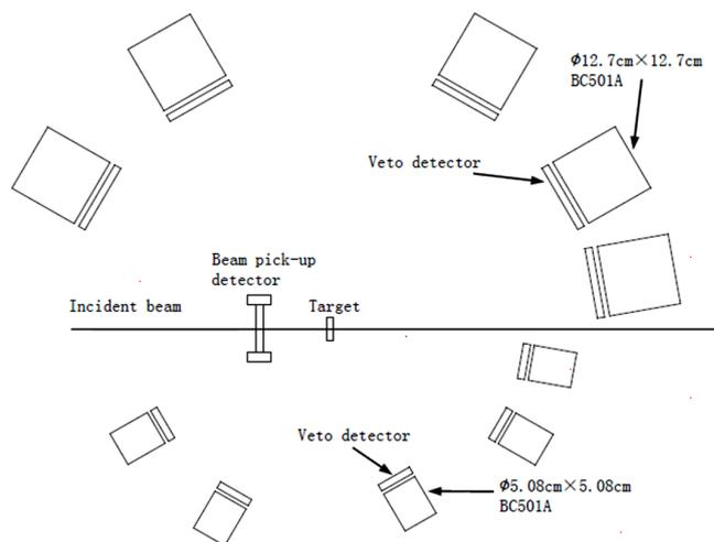
Fig. 3. A schematic view of the NTOF spectrometer.
