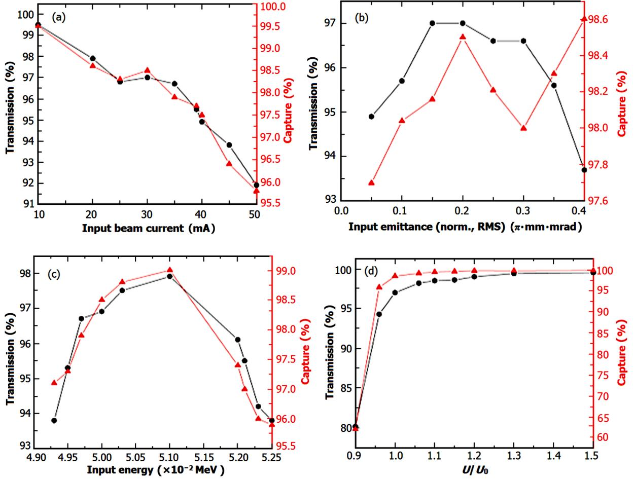
Fig. 4. (Color online) Effects of fluctuations in input beam current (a), input emittance (b), input beam energy (c) and intervane voltage (d) on transmission and capture according to the simulation results.
