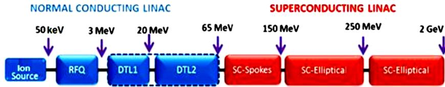
Fig. 1. (Color online) Block diagram of the TAC proton linac.
