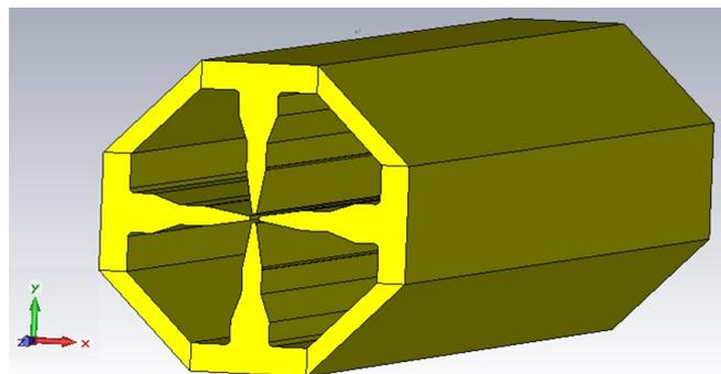
Fig. 7. (Color online) The three-dimensional unmodulated RFQ model.
