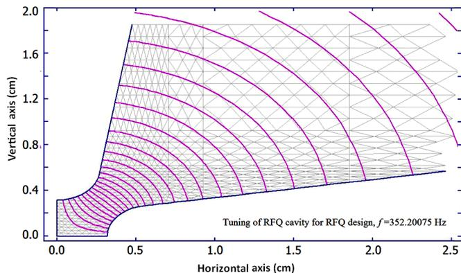
Fig. 6. (Color online) 2-D geometry of one quadrant of the RFQ electrodes obtained from SUPERFISH. The electric field pattern between the electrodes is indicated by lines.
