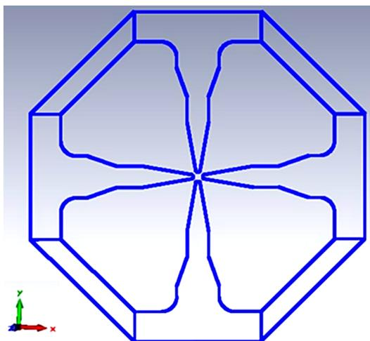
Fig. 5. (Color online) A full 2-D geometry of the RFQ electrodes constructed by CST MWS according to SUPERFISH results. The beam flows inward on  $z$ -axis.
