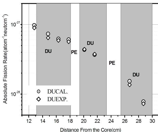
**Fig.4** Distribution of depleted uranium fission rates. (DUEXP represents experimental results. DUCAL represents calculated results)
