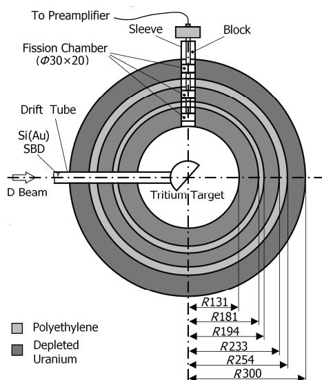
**Fig.1** Schematic diagram of the fission assembly
