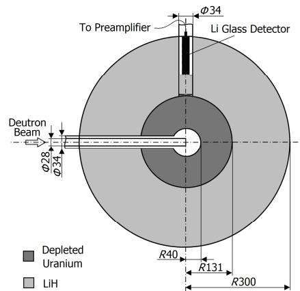
**Fig.2** Schematic diagram of the tritium production assembly.
