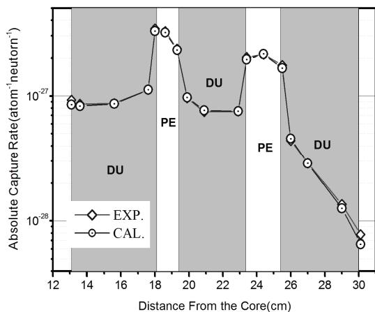
**Fig.3** Distribution of  $^{238}\text{U}$  capture reaction rates (DU, depleted uranium; PE, polyethylene)
