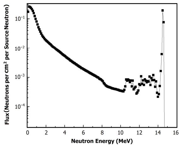
**Fig.6** Distribution of leakage neutron spectrum from the depleted uranium shell.
