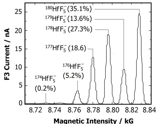
**Fig.2** The mass scan spectrum for  $\text{HfF}_5^-$  obtained in F3 Faraday cup. The relative intensities are very close to their natural isotopic abundances, indicating the lack of contaminating beams in the mass range covering  $\text{HfF}_5^-$  of all Hf isotopes.
