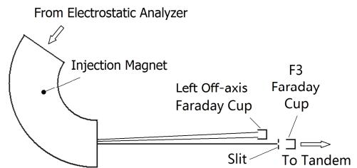
**Fig.1** Schematic setup for instantaneous monitoring of beam current for abundant reference nuclide in the measurement of  $^{182}\text{Hf}$ . (F3 Faraday cup is temporarily mounted for the measurement of  $^{180}\text{HfF}_5^-$  current  $I_{\text{F}3}$  and  $I_{\text{F}3}/I_{\text{oc}}$  only).
