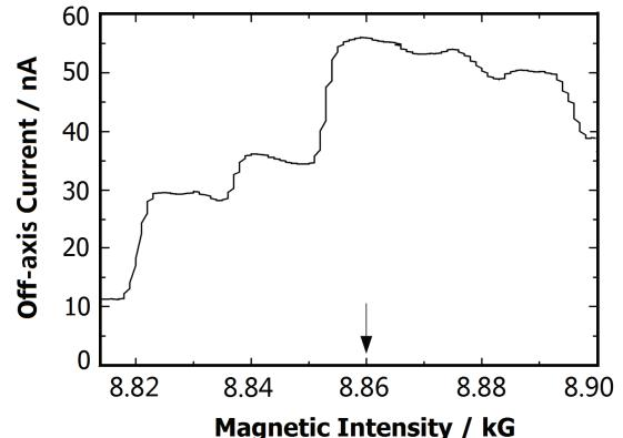
**Fig.3** Off-axis current vs magnetic strength. There is a flat part at the vicinity of 8.860 kG (corresponding to the magnetic rigidity of  $^{182}\text{HfF}_5^-$ ).
