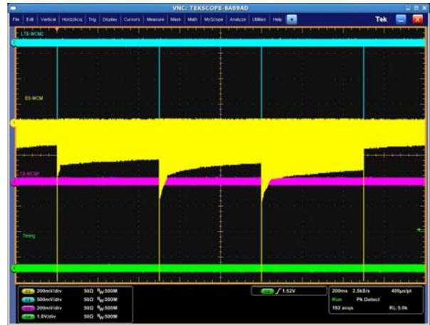
**Fig.3** Adjusted beam at 158 MeV, [8.18, 5.40], 200 mV/div.
