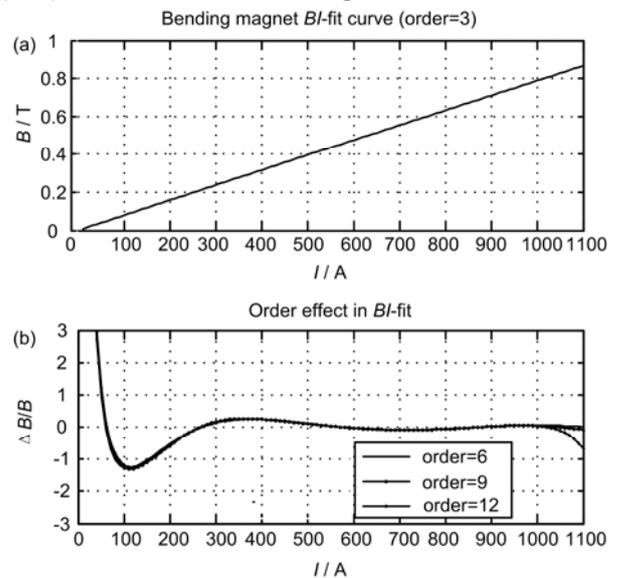
**Fig.1** Fitted  $B-I$  curve of BEND ( $n=3$ ) (a) and differences of fitted  $B-I$  curve in orders (b).
