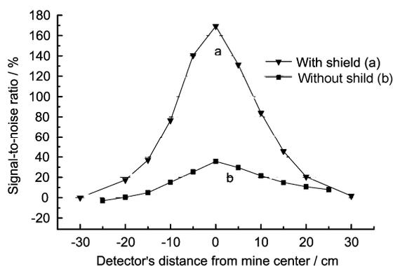
**Fig.6** Variation of signal-to- noise ratio with detector's distance from landmine center.
