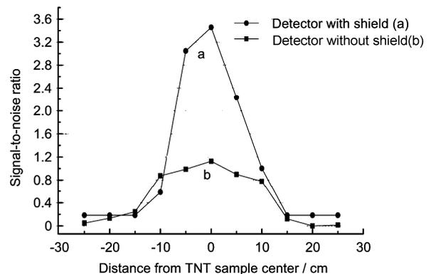
**Fig.3** Signal-to-noise ratio as a function of distance from center of buried TNT sample. a)Detector with two layers shields, boric acid thickness=4cm (outer layer) and PE thickness=10cm (internal layer). b)Detector without shield (MCNP code results).
