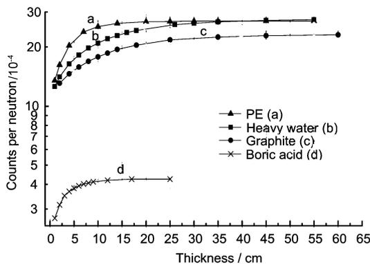
**Fig.4** Neutron population as a function of the moderator thicknesses.
