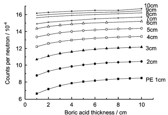
**Fig.5** Neutron flux as a function of boric acid thickness (second layer) for different thicknesses of PE (first layer).
