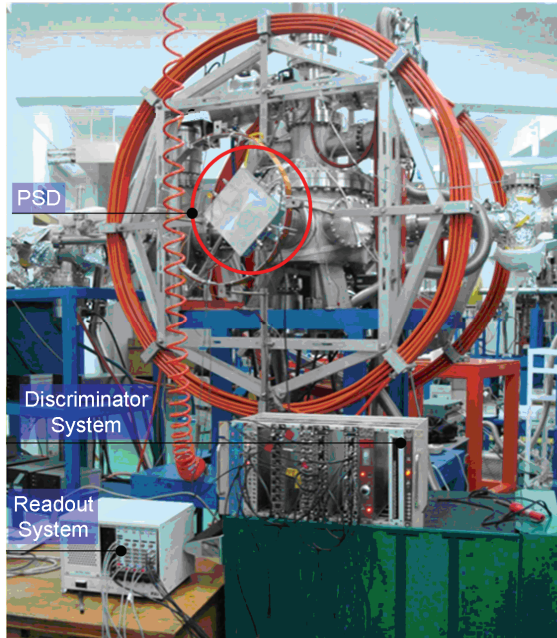
Fig.10 Readout system working with the COLTRIMS.
