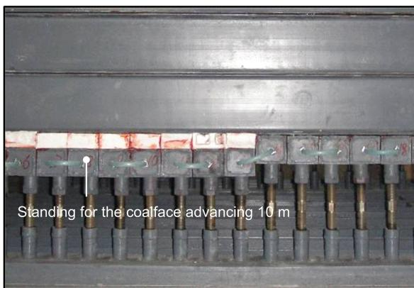
**Fig.3** Mining process simulation.
