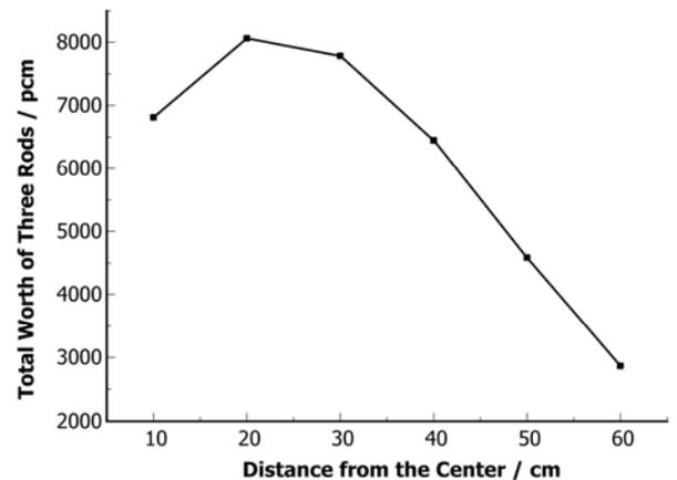
Fig.5 Total worth of three control rods varies with the radial position of control rods.
