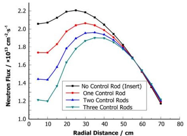
Fig.8 Radial neutron flux effect by the control rod.
