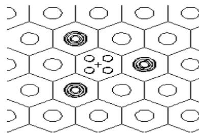
**Fig.1** Positions of control rods in reactor core.
