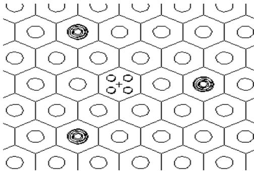
Fig.6 Positions of control rods after optimizing.
