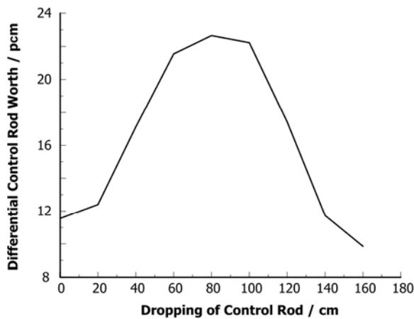
Fig.3 Differential worth of one control rod in TMSR (2 MW).
