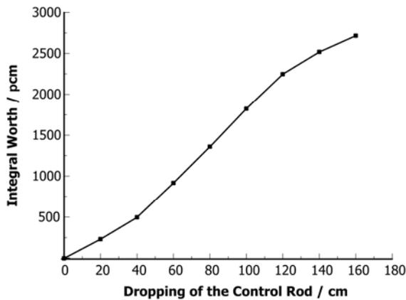
Fig.2 Integral worth of one control rod in TMSR (2 MW).
