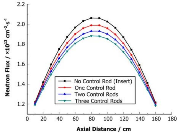
Fig.7 Axial neutron flux effect by the control rod.
