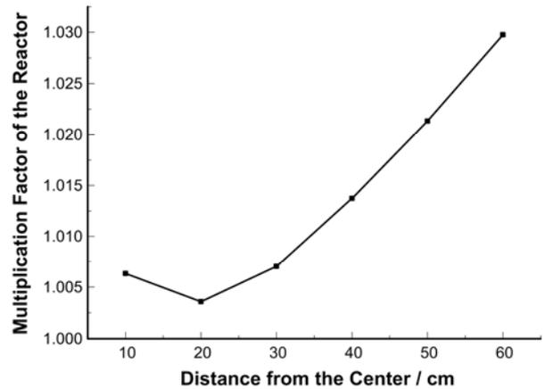
Fig.4 Multiplication factor varies with the radial position of control rods.
