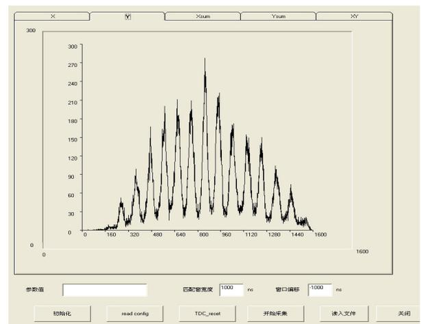
**Fig.1** A working space of the software. The abscissa is the time of flight, and the ordinate is the counts. It can show the TOF spectrum of each channel, or 2-dimensional position information.
