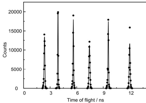
**Fig.2** Results of TDC. The time resolution of the TDC is 50 ps (FWHM).
