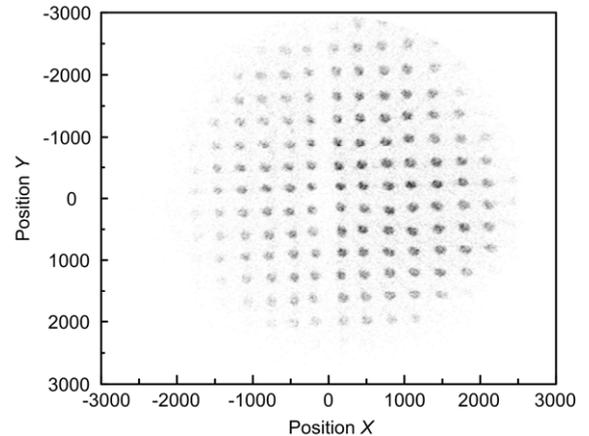
**Fig.3** Image of a shadow mask with an MCP detector of 75-mm active diameter.
