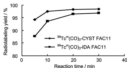
**Fig.5** Influence of heating time on the radiolabelling yields of  $^{99}\text{Tc}^{\text{m}}(\text{CO})_3\text{-CYST FAC11}$  and  $^{99}\text{Tc}^{\text{m}}(\text{CO})_3\text{-IDA FAC11}$  at 95 $^\circ\text{C}$ , pH=7.8.
