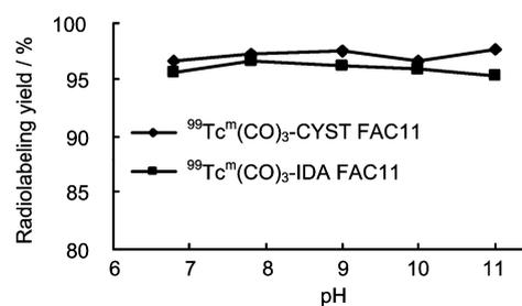
**Fig.3** Influence of pH value on the radiolabelling yields of  $^{99}\text{Tc}^{\text{m}}(\text{CO})_3\text{-CYST FAC11}$  and  $^{99}\text{Tc}^{\text{m}}(\text{CO})_3\text{-IDA FAC11}$  at 95 $^\circ\text{C}$ .
