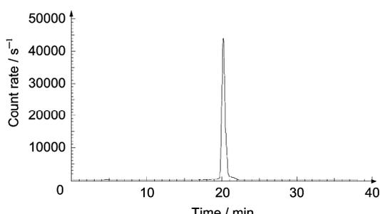
**Fig.1** Radio-HPLC chromatograms of  $^{99}\text{Tc}^{\text{m}}(\text{CO})_3\text{-CYST FAC11}$ .
