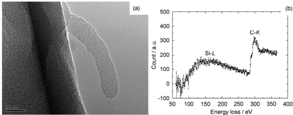
**Fig.4** Bright-field TEM image (a) and typical EELS spectra (b) of the CNW.
