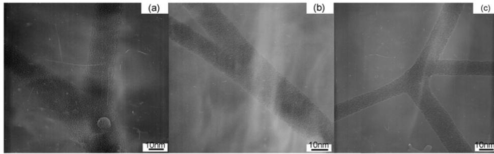
**Fig.3** HRTEM images of CNJs in “Y” (a), compressed “Y” (b), or “K” (c) shape.
