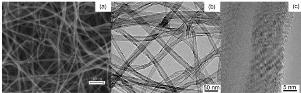
**Fig.1** Typical morphology and structure of the as-grown CNTs. (a) SEM image, (b) TEM image, (c) HRTEM image.
