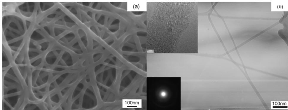
**Fig.2** Typical SEM and TEM images of the CNTs irradiated with 40 keV Si ions to a dose of  $1 \times 10^{17} \text{ cm}^{-2}$ . (a) SEM image, (b) TEM image. The insets are HRTEM (upper left) and SAD (low left) images.
