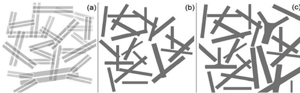
**Fig.5** Schematic processes of the CNJs synthesis. (a) As-grown CNTs, (b) Defect generation to form amorphous region, (c) Formation of CNJs with different shapes.
