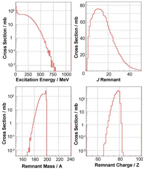
**Fig.5** (Color online) The  $E^*$ ,  $J$ ,  $A$  and  $Z$  distributions of residual nuclei populated in (1 GeV)  $p+^{200}\text{Hg}$  collisions predicted by the INCL model<sup>[25]</sup>.
