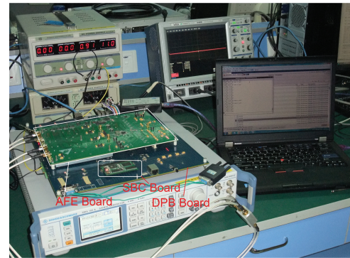
Fig.10 The DBPM system in laboratory test.
