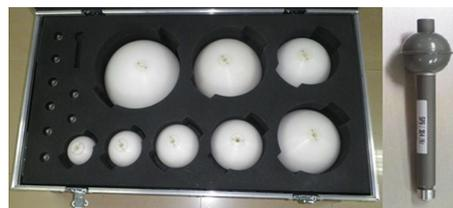
**Fig. 1** Eight PTB polyethylene spheres and SP9  $^3\text{He}$  proportional counter
