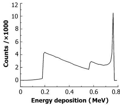
**Fig. 4** Energy deposit spectrum of the  $^3\text{He}$  proportional counter. *Peak 1* is a full collection of the energy deposition of 0.2 MeV triton; *peak 2* was contributed by the full collection of the energy deposition of 0.57 MeV protons; and *peak 3* is the whole energy peak with total collection of the energy deposition of 0.2 MeV triton and 0.57 MeV proton
