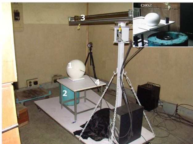
**Fig. 2** Measurement assembly. 1 PE sphere, 2 <sup>241</sup>Am-Be neutron source, 3 source-lifting mechanism and 4 coaxial cable
