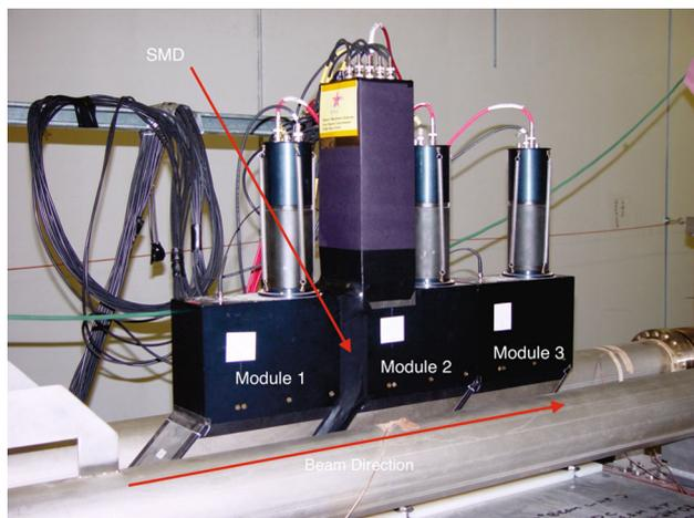
**Fig. 2** ZDC modules installed on RHIC-STAR experiment
