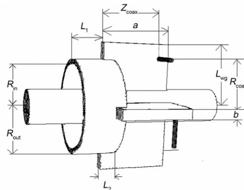
**Fig. 7** Structure of vacuum part of BPM. The parameters (in mm) are:  $R_{\text{in}}$ , 44.000;  $R_{\text{out}}$ , 47.900;  $L_1$ , 30.304;  $L_2$ , 10.000;  $a$ , 70.000;  $b$ , 10.000;  $L_{\text{wg}}$ , 65.000;  $Z_{\text{coax}}$ , 55.060; and  $R_{\text{coax}}$ , 55.050.
