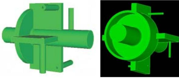
**Fig. 3** Cut-through waveguide and re-entrant cavity.
