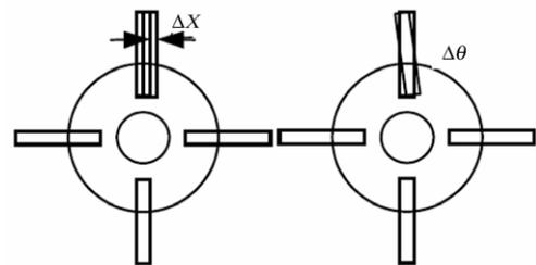
**Fig. 10** Waveguide misalignment.
