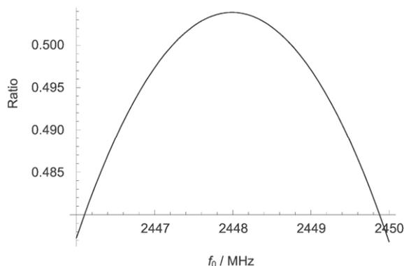
**Fig. 5** Ratio between effective energy loss and total energy loss vs.  $f_0$ .
