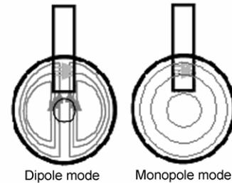
Fig. 2 Sketch of dipole mode and monopole mode.
