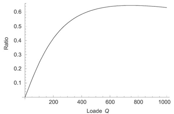
**Fig. 4** Ratio between effective energy loss and total energy loss vs. loaded  $Q$ .
