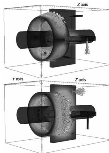
**Fig. 6** Two orthogonal dipole modes, simulated by Omega3p.
