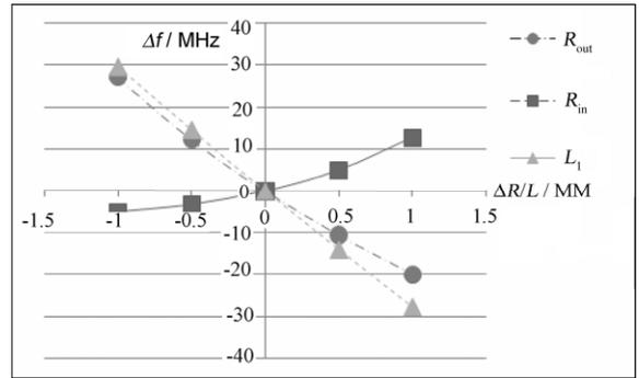
**Fig. 9** External  $Q$  variations of TM110 mode with waveguide size.
