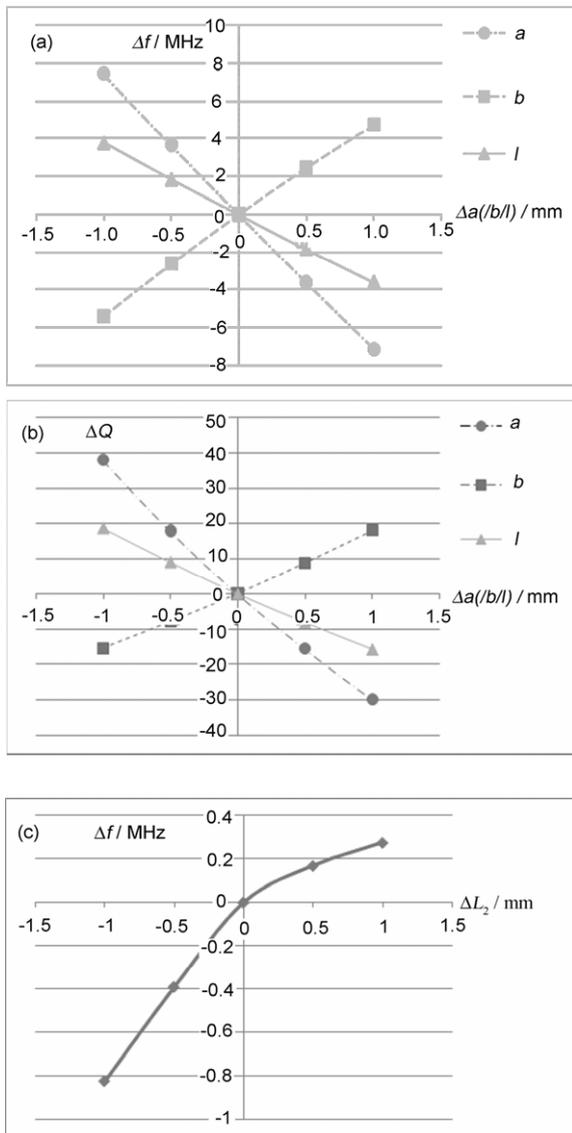
**Fig. 8** Frequency variations of TM110 mode with the waveguide size (a), and the cavity shape (b) and thickness (c).
