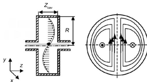
Fig. 1 Sketch of pick-up station and dipole mode.
