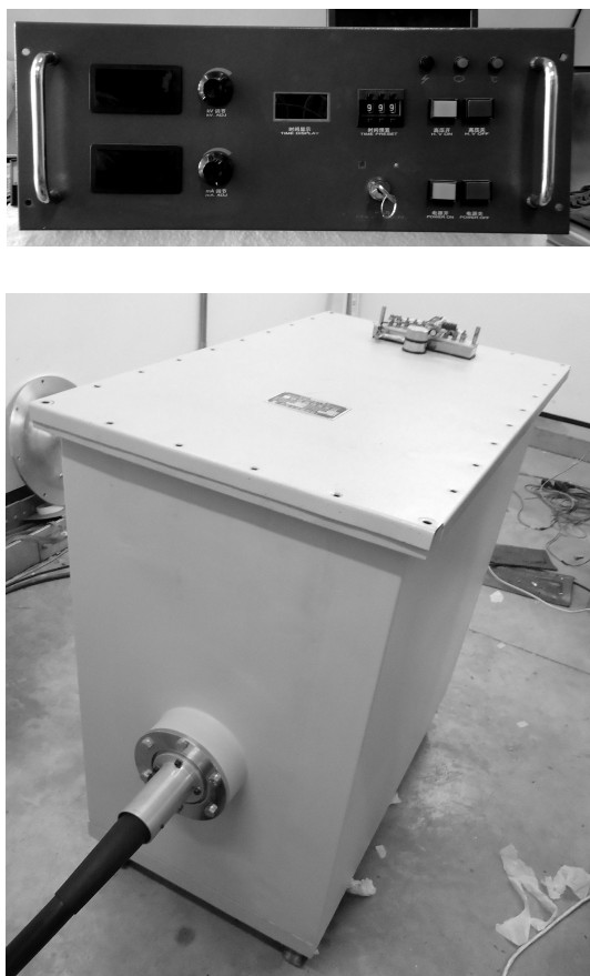
Fig.2 200 kV/20 mA high voltage power supply.
