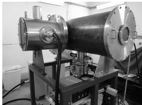
Fig.3 Electron curtain accelerator.
