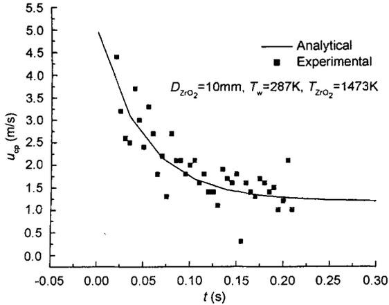
**Fig.3** The  $u_{cp}$  of 10 mm  $ZrO_2$  particle obtained from experimental data and those predicted by the HPMC model.
