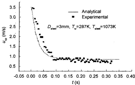
**Fig.5** The  $u_{cp}$  of 3 mm steel ball obtained from experimental data and those predicted by the HPMC model.
