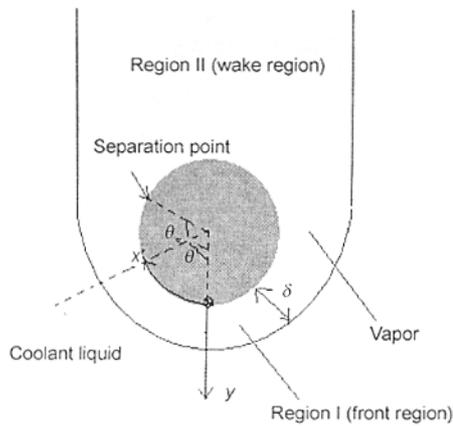
**Fig.1** Scheme of a high-temperature particle moving in coolant liquid.
