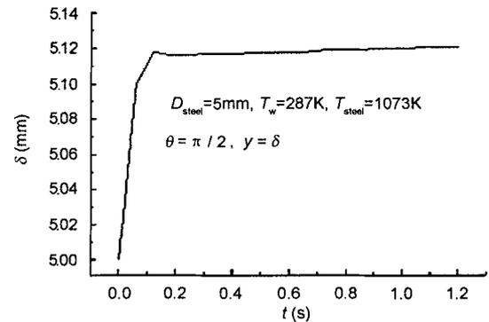
**Fig.7** The transient process of film thickness calculated by the HPMC model.
