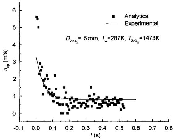
**Fig.4** The  $u_{cp}$  of 5 mm  $ZrO_2$  particle obtained from experimental data and those predicted by the HPMC model.
