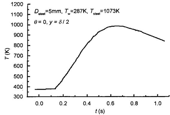
**Fig.6** The transient process of temperature calculated by the HPMC model.
