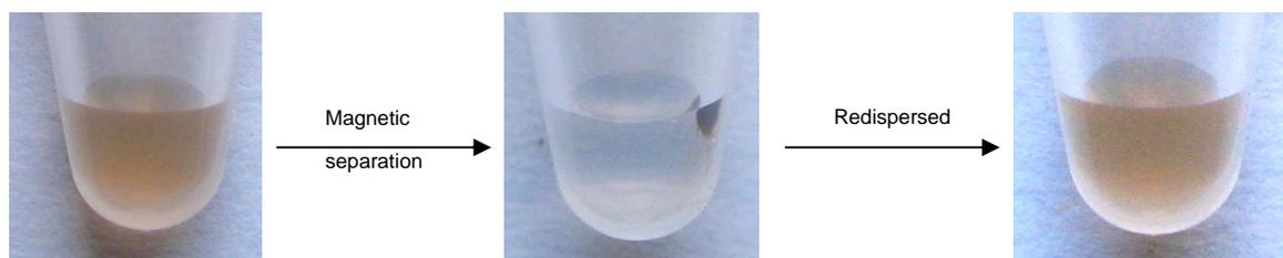
**Fig. 3** Amino-MNPs separated by magnet and redispersed. Observations on stability of the amino-MNPs show that placing them at 4°C for over one month, the particles were easily dispersed with gentle shaking.
