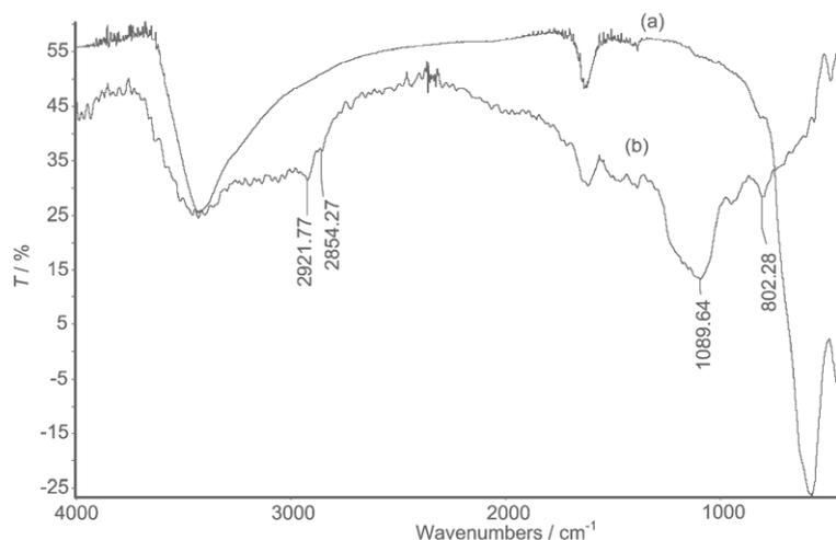
**Fig. 4** FT-IR spectra of naked (a) and coated (b) MNPs.
