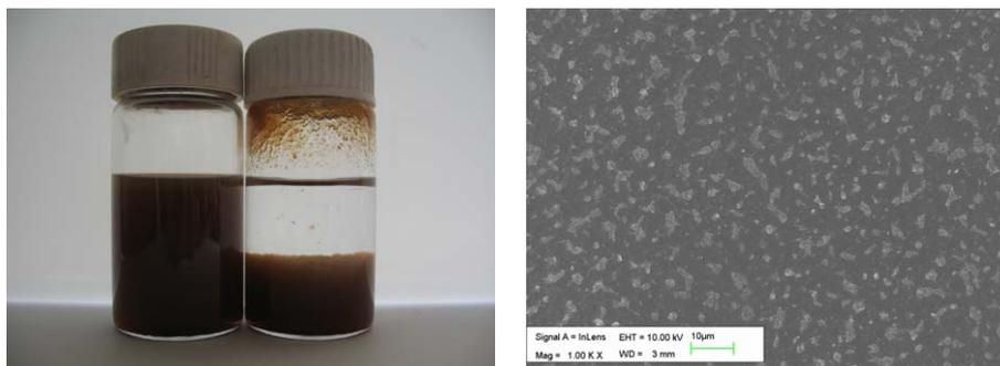
**Fig. 2** Magnetic fluids prepared by sonication (left) and stirring method (right), after 1h placing at RT.
