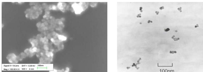
**Fig. 1** SEM (left) and TEM (right) images of naked MNPs. The MNPs were well-distributed spherical particles of  $\phi 10\sim 15$  nm.
