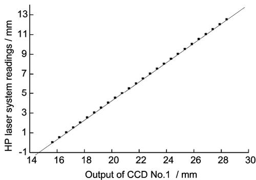
**Fig.5** Calibration results of CCD No.1.
