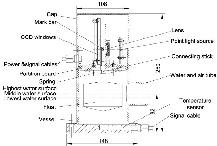
**Fig.1** Cross section of the HLS vessel.
