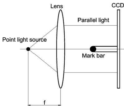
**Fig.2** Light, mark bar and CCD system.
