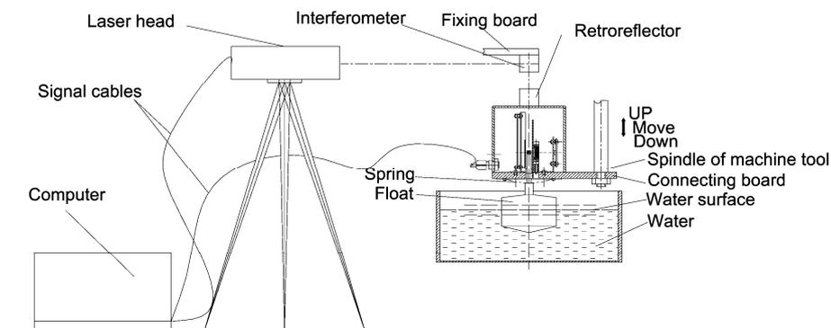
**Fig.6** Calibration system for one vessel.
