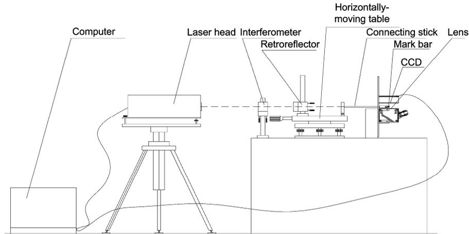
**Fig. 4** Layout of the CCD calibration system.
