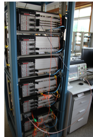
Fig. 6. (Color online) Offline test platform of the timing system.
