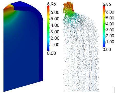
Fig. 12. (Color online) Velocity field in the core ( $U/m \cdot s^{-1}$ ).
