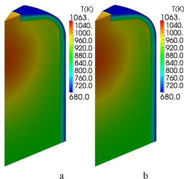
Fig. 22. (Color online) Temperatures with convective term (a), with convective and turbulent diffusion term at  $Sc_t = 0.7$  (b).
