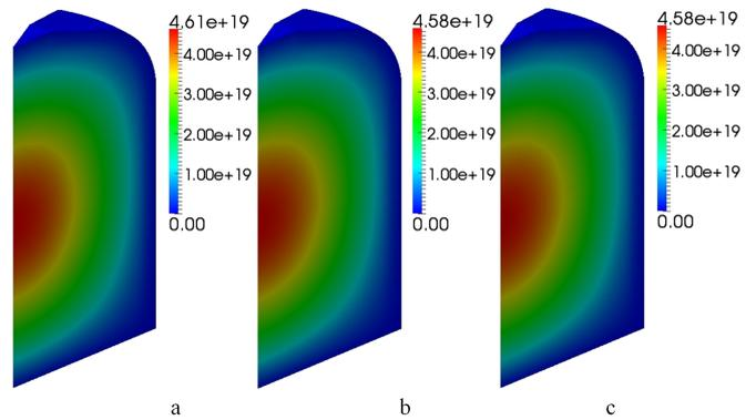
Fig. 14. (Color online) Fast neutron fluxes without flow (a), with convective term (b), with convective and turbulent diffusion term at  $Sc_t = 0.7$  (c) (Unit/neutron  $\cdot m^{-2} \cdot s^{-1}$ ).
