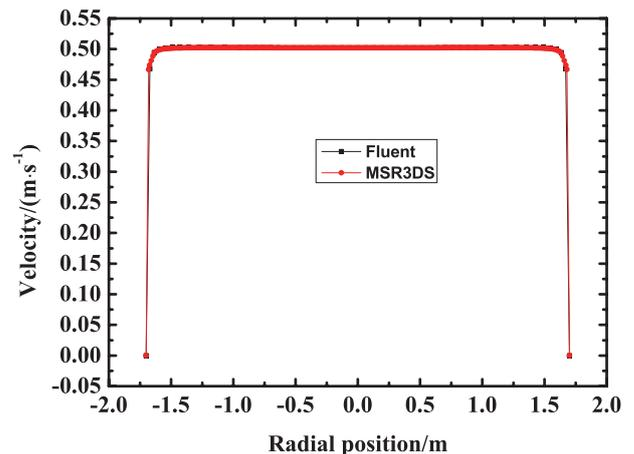
Fig. 9. (Color online) Velocities along radial direction at the mid-plane.
