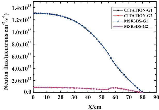
Fig. 5. (Color online) Distributions of the neutron fluxes calculated by CITATION and MSR3DS at (Z=79.2 cm, Y=40 cm).
