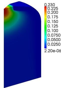
Fig. 13. (Color online) Turbulent kinematic viscosity in the core ( $\nu_t/m^2 \cdot s$ ).
