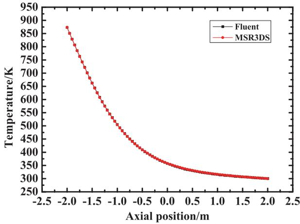
Fig. 10. (Color online) Temperatures at the symmetry axis.
