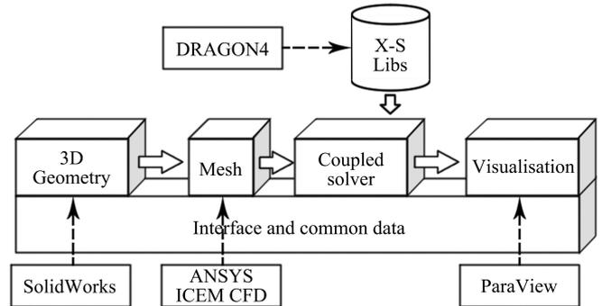
Fig. 4. The program diagram of the MSR3DS code.
