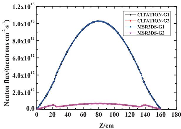
Fig. 6. (Color online) Distributions of the neutron fluxes calculated by CITATION and MSR3DS at (X=40 cm, Y=40 cm).
