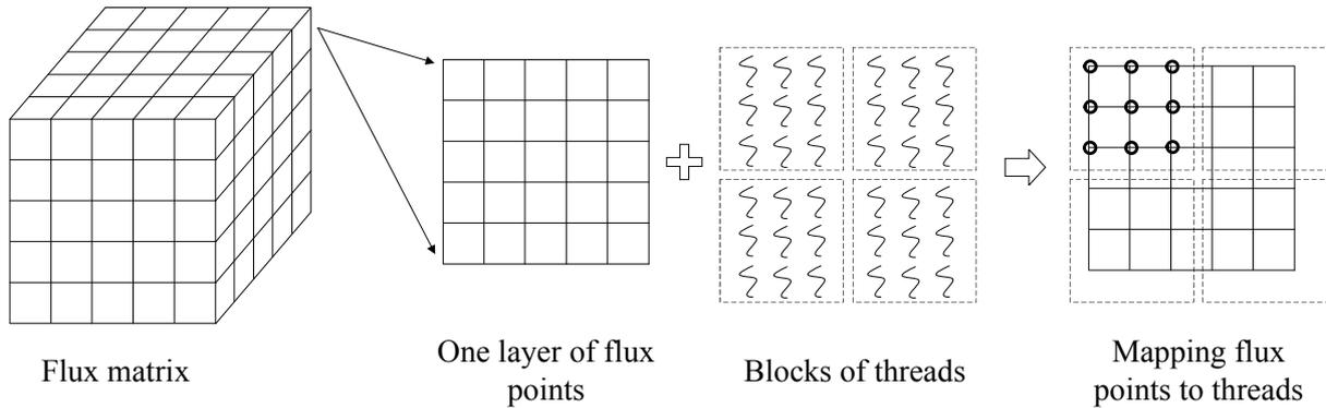
Fig. 2. Mapping relationships between flux points and threads.
