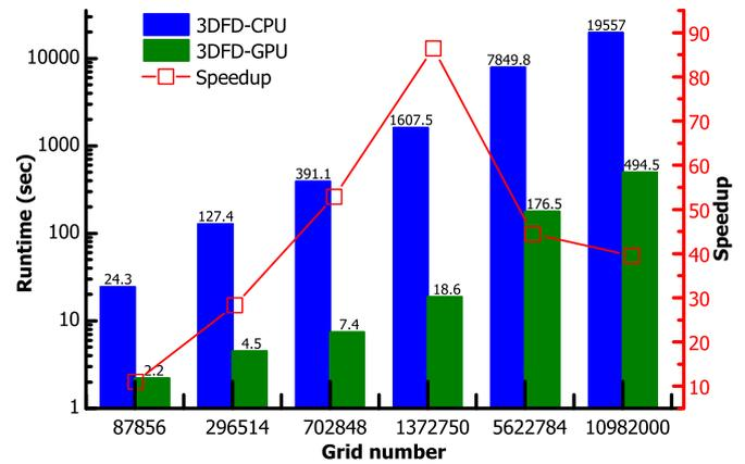
Fig. 5. (Color online) Performance comparison between 3DFD-GPU and 3DFD-CPU.
