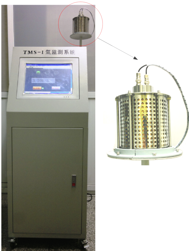
Fig. 3. (Color online) The TMS-I tritium-in-air monitor.
