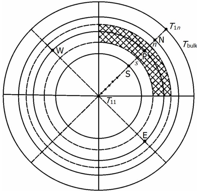
Fig. 1. Mesh layout of the heat structure.
