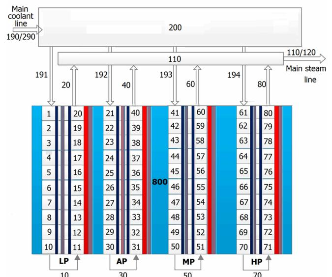
Fig. 5. (Color online) SCTRAN idealization of Canadian-SCWR concept. The control volumes are numbered as 1–80.
