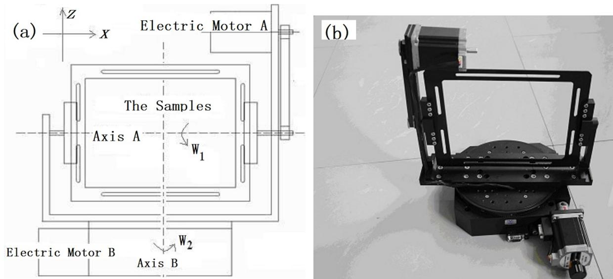
Fig. 7. (Color online) (a) The schematic representation and (b) the picture of the biaxial rotational equipment.
