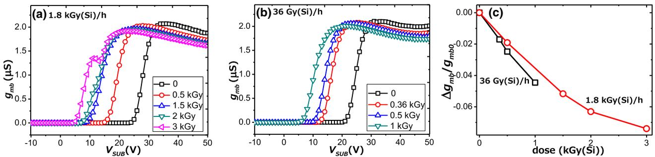
**Fig. 5** (Color online) Transconductance of back gate at different TIDs at high (a) and low (b) dose rates, and the normalized maximum transconductance (c)
