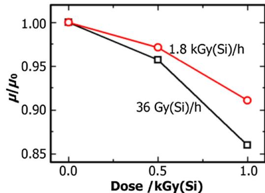
Fig. 3 (Color online) Normalization mobility as a function of irradiation dose under different dose rates
