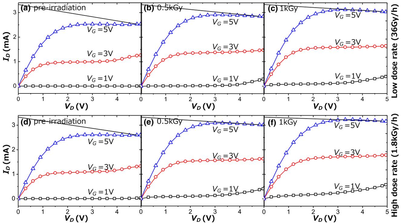
Fig. 2 (Color online)  $I_D$ – $V_D$  curves of front gate as a function of radiation dose at different dose rates
