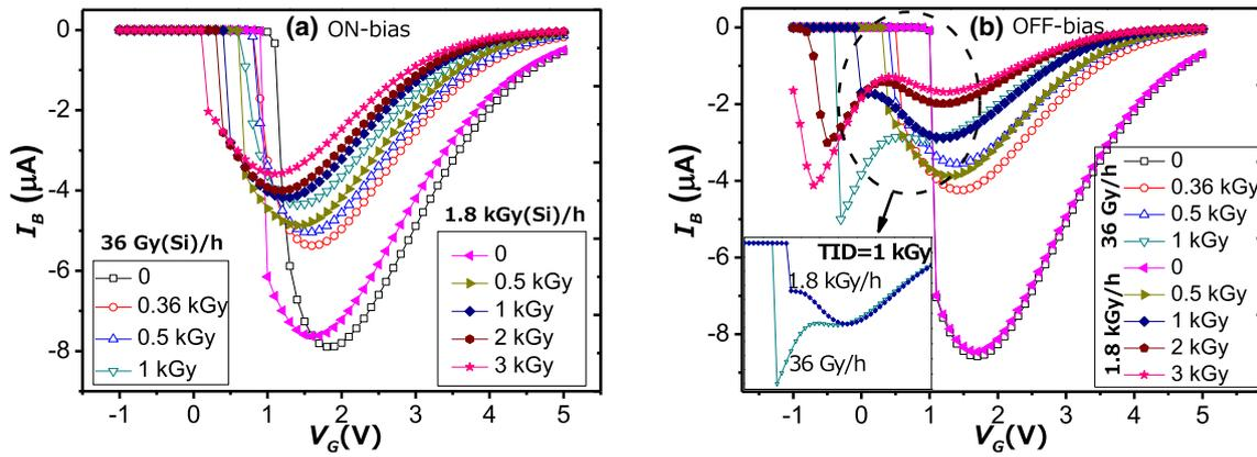
**Fig. 4** (Color online)  $I_B$ – $V_G$  curves before and after irradiation for ON-bias (a) and OFF-bias (b)
