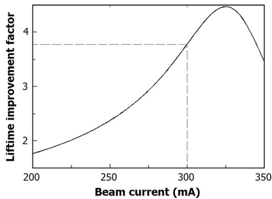
**Fig. 1** Lifetime improvement factor versus beam current for the SSRF storage ring
