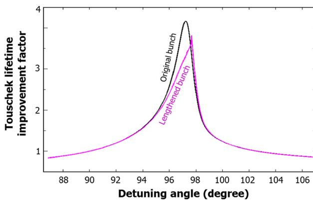
Fig. 5 (Color online) The lifetime improvement factors before and after using iteration method with lengthened bunch
