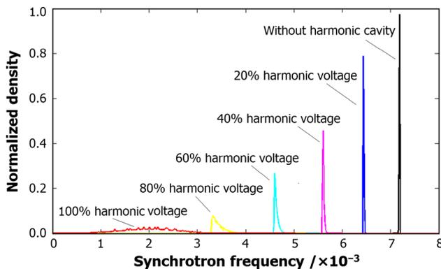
Fig. 6 (Color online) Synchrotron frequency spread for various harmonic voltages in SSRF case
