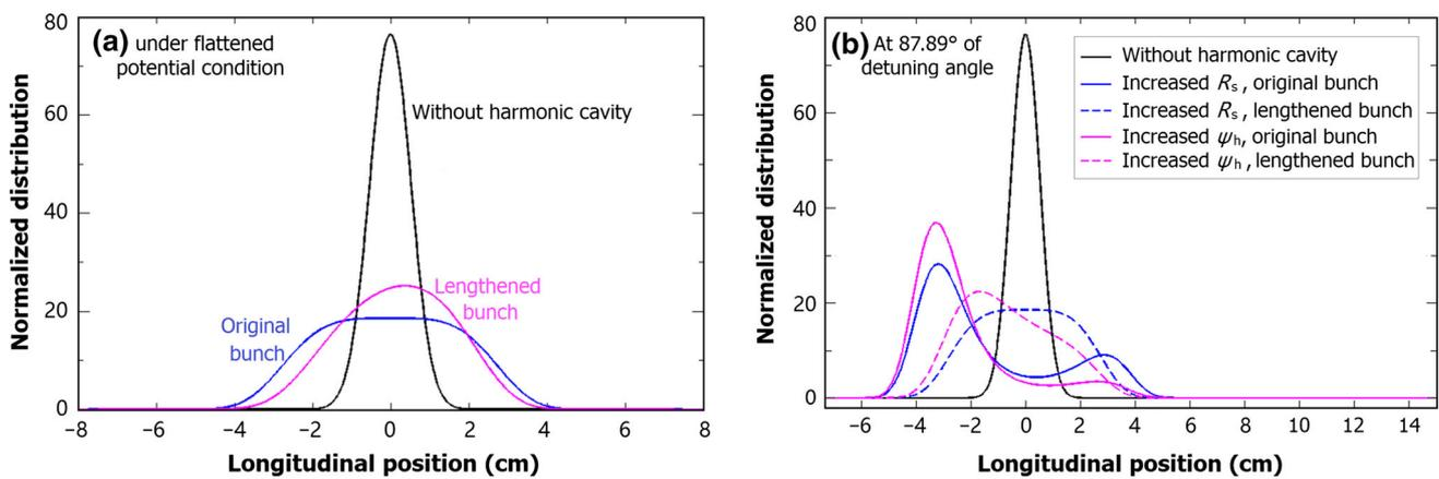
Fig. 4 (Color online) The bunch distributions under the flattened potential condition (a) and 87.89° detuning angle (b)
